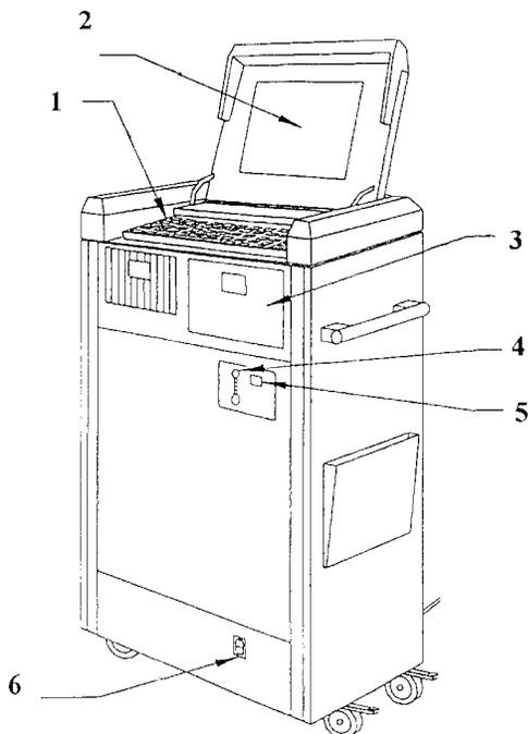
Fig. 3. OBS/L system for optical biopsy (USA): 1) keyboard; 2) display; 3) disk drives; 4) optical fiber adapter; 5) radiation power meter; 6) power switch.
